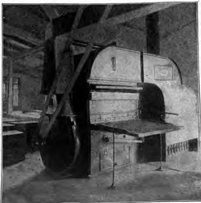
DRYING TEA BY A HOT BLAST.
